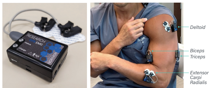
Figure 2. Wireless EMG electrodes recorded muscle activity from five muscle groups on the surgeon's working arm. Flexor carpi radialis sensor not pictured.
