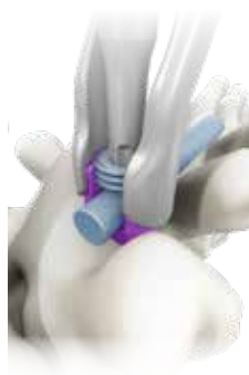
Figure 5 Closure top introduced to hook, with angled hook holder attached
